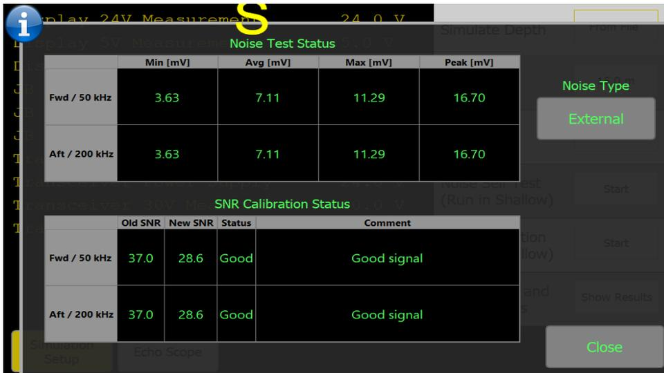
The values shown should be below 20mV once installed unless otherwise stated. High values can usually be reduced by improved cabling and / or filters on the power supply.
