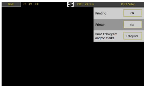
When the printer is first set to ON on the display, a Test/Title page will be printed. This can be used to test the setup is correct.
